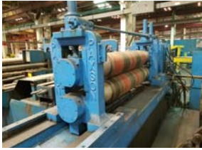
Stock #VX-1600 60" x .187" x 50,000 Lb. Paxson Slitting Line, 8" Arbor, 2 Heads
