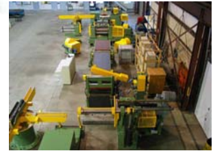
Stock #VX-1492 36" x .135" x 30,000 Lb. Alcos Slitting Line, 6" Arbor, 2 Heads
