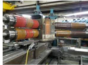
Stock #VX-1597 72" x .375" x 70,000 Lb. Braner Slit Line, 9.5" Arbor, 3 Heads
