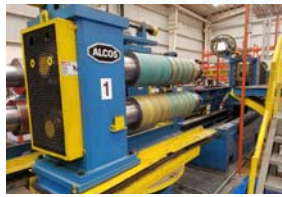
Stock #VX-1558 60" x .187" x 50,000 Lb. Alcos Slitting Line, 8" Arbor 2 Heads
